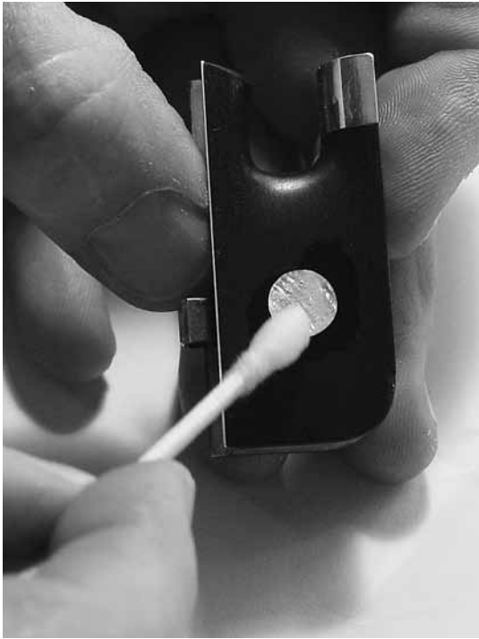
Fig. 7 Hydrochloric acid is applied with a cotton swab to dissolve excess pearl.
